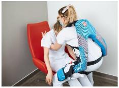
MUSCLE SUIT Every is a work-assisting robotic suit that lightens the load on the user's back when the user performs hard work, such as maintaining a half-crouching position and lifting up a heavy item or person. The powered
